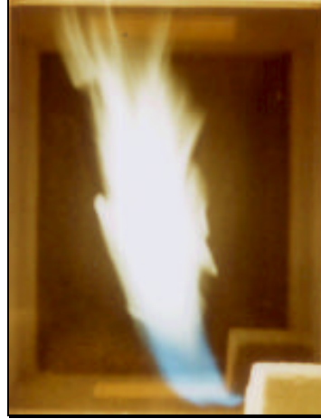
Fig.7. Flame photographs with combustion air temperature of 1100^{\circ}\text{C} and oxygen concentration of 21%, 8% and 2%
