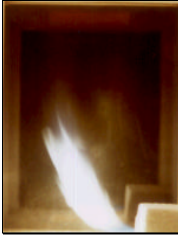
Fig.7. Flame photographs with combustion air temperature of 1100^{\circ}\text{C} and oxygen concentration of 21%, 8% and 2%
