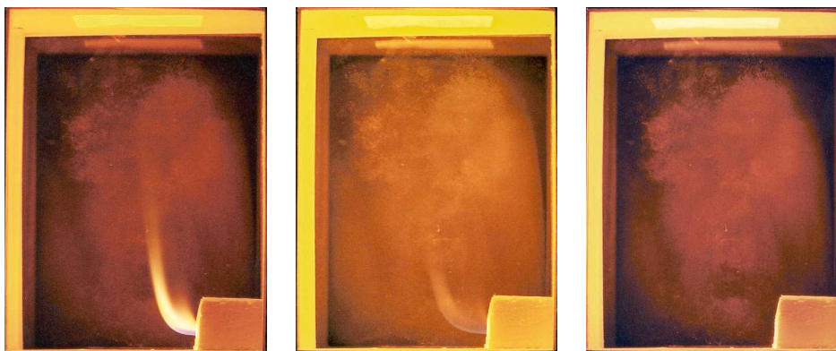
Fig 14. Hydrogen flame photographs with combustion air temperature of 1000°C and oxygen concentrations of 21%, 8% and 2%, respectively (dilution gas: Nitrogen).
